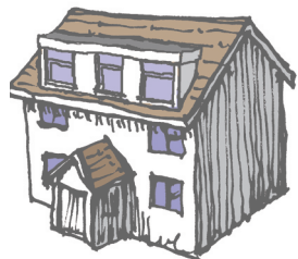
Typical Flat Roof, Full Width
